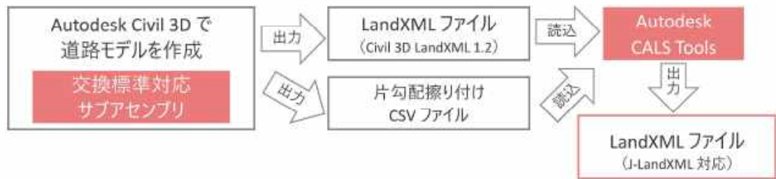
図 11.2 AutoCAD Civil3D での J-LandXML 変換
